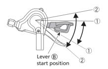
"The gears can be shifted by either pushing or pulling the lever."
